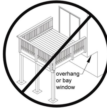
Figure 18: No Attachment to House Overhang
